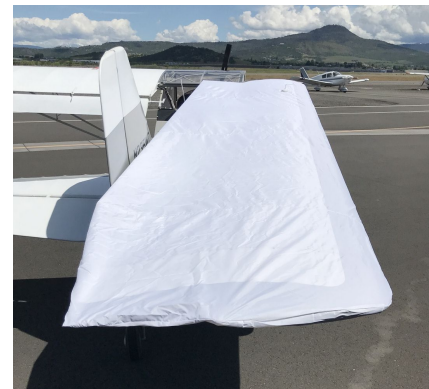
Kitfox Wing Covers, Folded Wing Type, test fit cover
