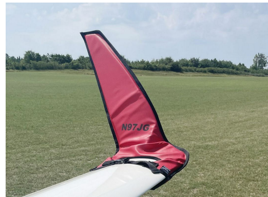
Schempp-Hirth Ventus-2B winglet/wingtip pads
