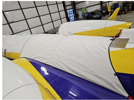
Lear 45 Empennage Saddle Cover W/ Dorsal Inlet Plug (Covers Upper Fuselage Between Pylons, Acm/Apu Area)
