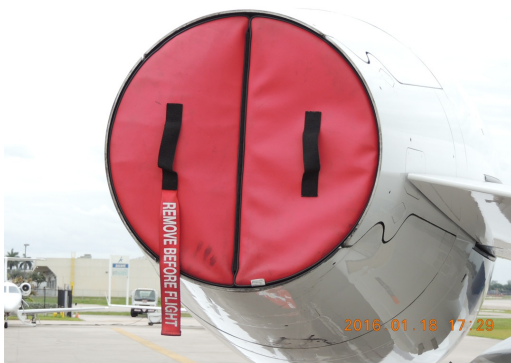
Embraer Legacy 500 Engine Exhaust Plug, folding type
