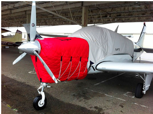
Beech Bonanza Insulated Engine Cover, fully enclosed
