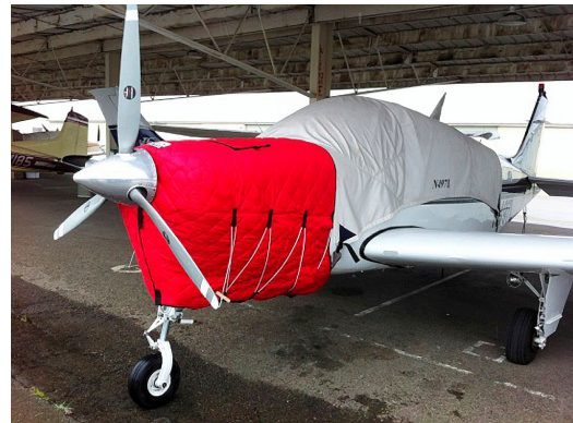
Beech Bonanza Insulated Engine Cover, fully enclosed
