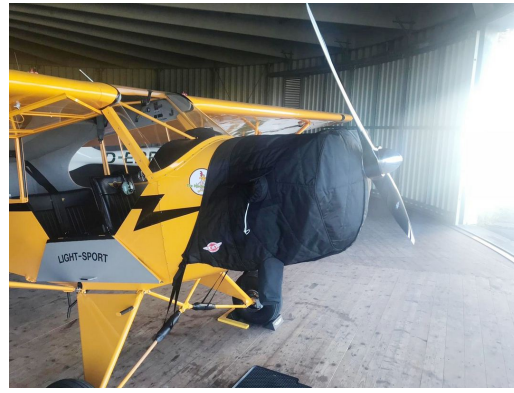
Legend Cub AL3 Insulated Engine Cover with special preheater access vent and attachment detail and fully enclosed under cowling.
