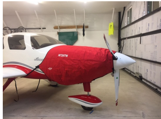
Lancair ES Insulated Engine Cover, Fully Enclosed
