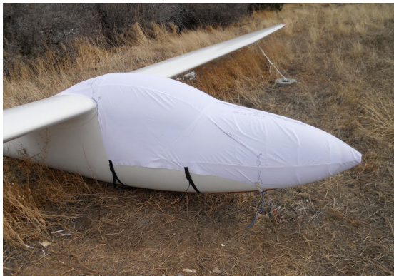
Laister LP-49 Canopy/Nose Cover, test fit cover
