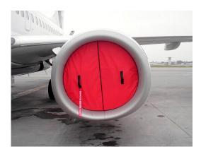
Boeing 737 Engine Intake Plug, Folding Type
