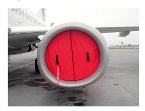
Boeing 737 Engine Intake Plug, Folding Type
