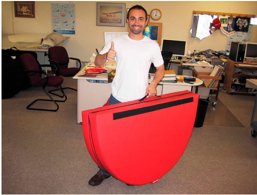
Boeing 737 FOD protection Intake Plug, folding type
