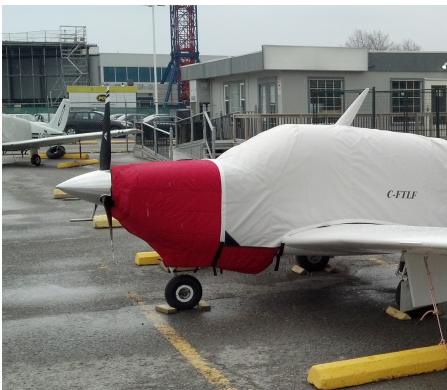
Mooney 201 Insulated Engine Cover, fully enclosed
