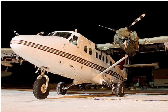
Twin Otter Wing, Horiz. Stab & Engine Covers De Havilland Twin Otter Insulated Engine & Insulated Propellor/Spinner Covers
