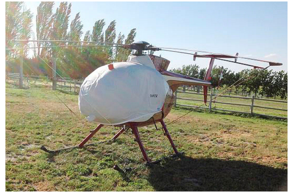
MD500D Bubble Cover with Intake Add-On
