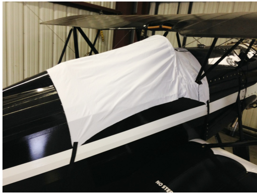
Rose Parrakeet Canopy Cover (test fit cover)
