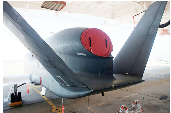
RQ-4/MQ-4 Global Hawk Exhaust Plug w/ lip (Fits both A & B models & all blocks)
