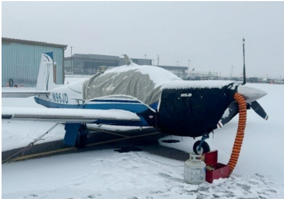
Mooney Bravo Insulated Engine Cover, Fully Enclosed
