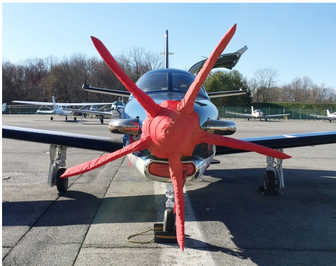
Socata TBM Insulated 5-Blade Prop/Spinner Cover
