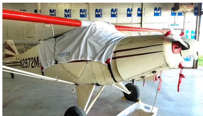
Piper PA-12 Wrap-Around Canopy Cover, Engine Plugs
