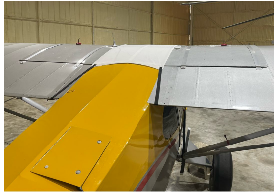
Piper J5A Windshield/Skylight Cover, test fit
