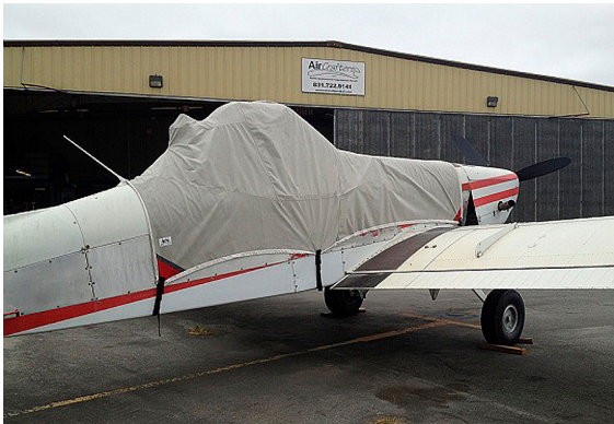
Piper Brave PA-36 Canopy/Hopper Cover
