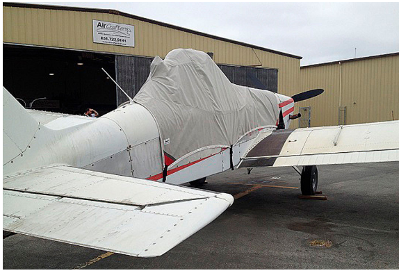
Piper Brave PA-36 Canopy/Hopper Cover
