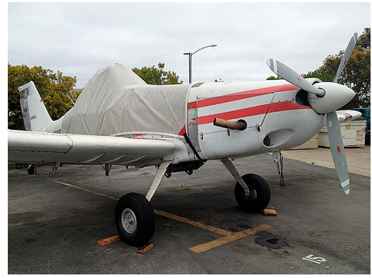
Piper Brave PA-36 Canopy/Hopper Cover
