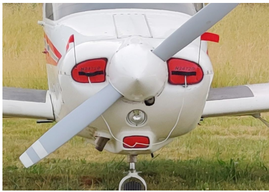
Piper PA-38 Tomahawk Engine Plugs
