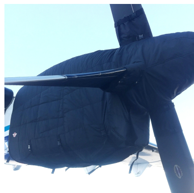
ATR-72-202 Insulated Engine & Prop Hub Covers
