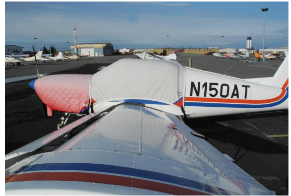
Koliber 150A Canopy Cover, Insulated Engine Cover
