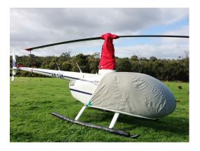
Robinson R-44 Bubble, Rotor Hub, Tail Rotor Covers, & Blade Tie-Downs
