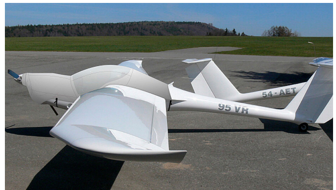
Lambda Canopy/Engine Cover (illustration)
