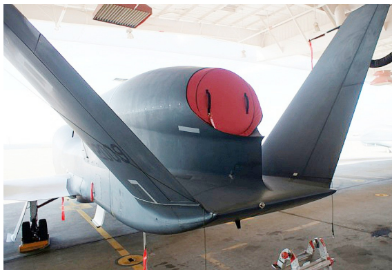
RQ-4/MQ-4 Global Hawk Exhaust Plug w/ lip (Fits both A & B models & all blocks)
