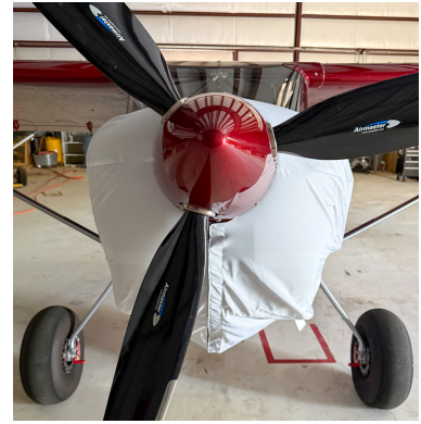
Rans S-21 Engine Cover, test fit cover
