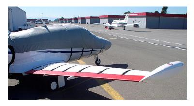
Fuselage Cover with Hail Protection & Wing Control Surfaces Hail Protection Pads
