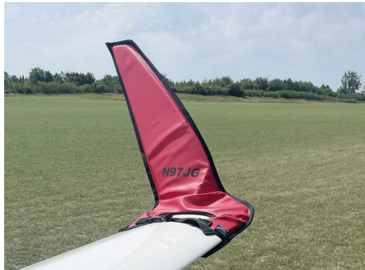
Schempp-Hirth Ventus-2B winglet/wingtip pads
