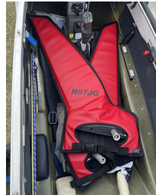
Schempp-Hirth Ventus-2B winglet/wingtip pads
