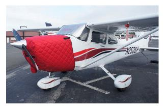
Cessna 172 Insulated Engine Cover, fully enclosed
