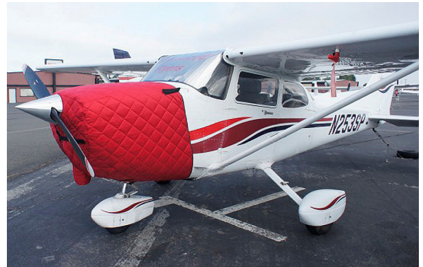
Cessna 172 Insulated Engine Cover, fully enclosed
