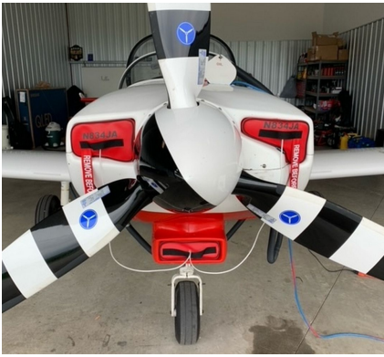
Slingsby T-67 Firefly Engine Inlet Plugs ENGINE PLUGS PREVENT BIRD NEST FOD. Piper Saratoga Engine Cowling Bird's Nest
