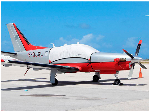
TBM Canopy Cover, Prop Tie/Exhaust Covers
