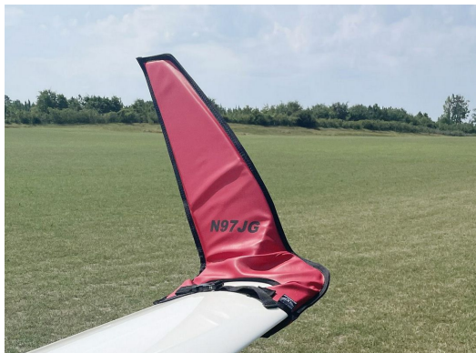
Schempp-Hirth Ventus-2B winglet/wingtip pads
