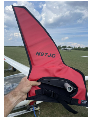
Schempp-Hirth Ventus-2B winglet/wingtip pads
